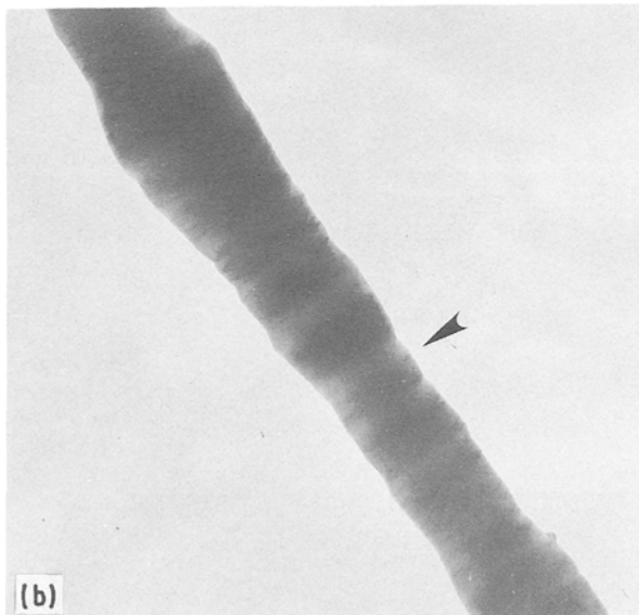
Figure 2 (a) The geometry and surface morphology of SiC whiskers. (b, c) Transmission electron micrographs showing stacking faults on the whiskers in bright and dark field \times 26000 .
